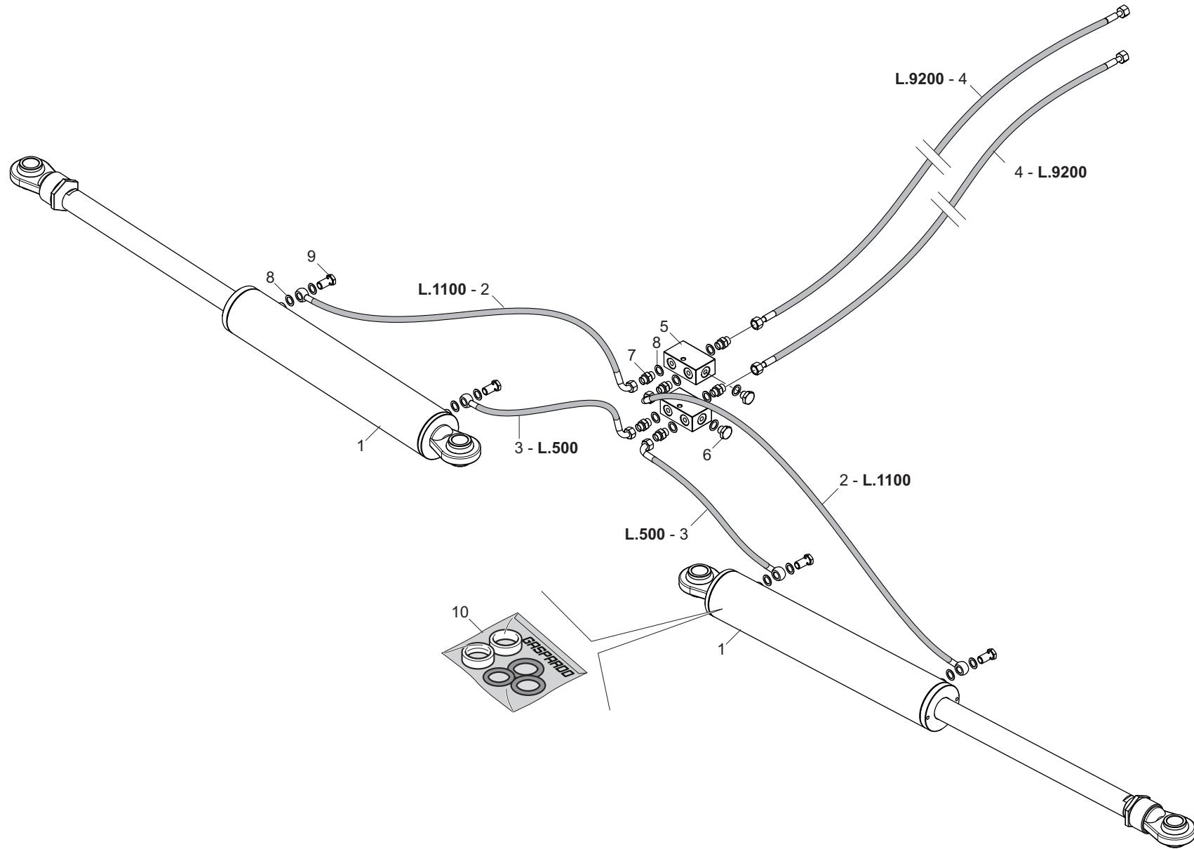
**IMPIANTO IDRAULICO ALI LATERALI / HYDRAULIC SYSTEM OF THE SIDE SECTIONS /
