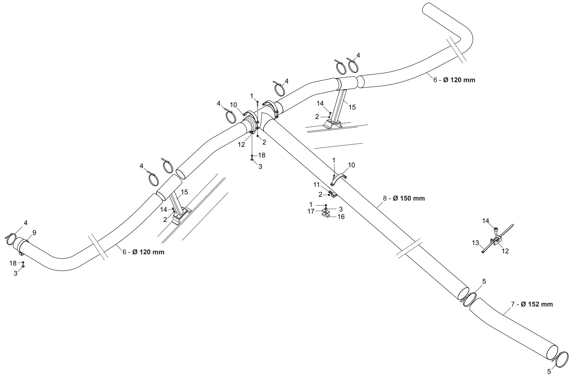
**TUBI TRASPORTO ARIA / AIR TRANSPORT PIPES / LUFTVERKEHR ROHRE /
