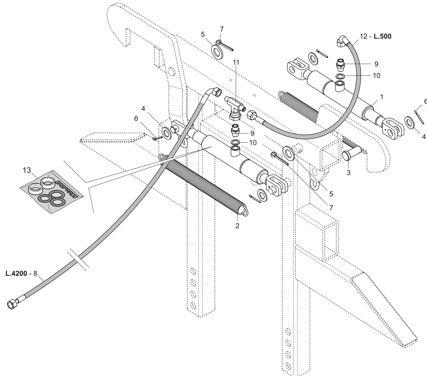
**IMPIANTO IDRAULICO BLOCCAGGIO LATERALI / HYDRAULIC SYSTEM THE SAFETY DEVICE OF THE SIDE
