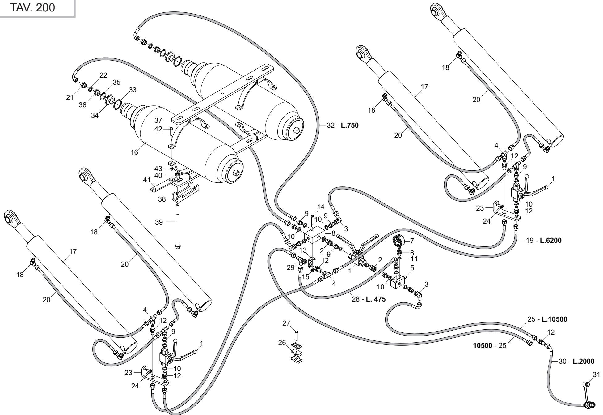
**IMPIANTO IDRAULICO SOLLEVATORE / HYDRAULIC LIFT**
